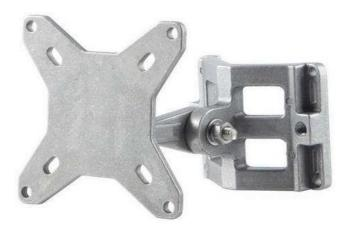
At last, it's a universal mounting bracket that is suitable for most UHF RFID antennas and mounting options, which includes mast mount and wall mount. It 's easy to mount with UDLR (up, down, left and right) adjustable clamp and tilts. There is no limit for the diameter of the mounting mast/pole. It ranges from 38mm to 100mm or more significant with optional 304 stainless steel adjustable clamps.
