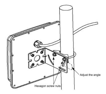
Step 4: Use an M6 wrench or suitable adjustable wrench to tighten the assembly to the mast. Tighten the hex nuts evenly. Do not over tighten
